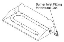
Figure 15 - Remove Burner Inlet FItting
